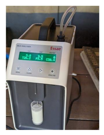
Figure 2: Milk analyzer
