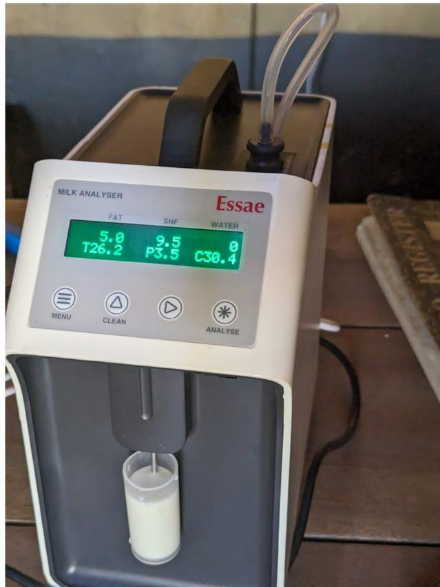
Figure 2: Milk analyzer
